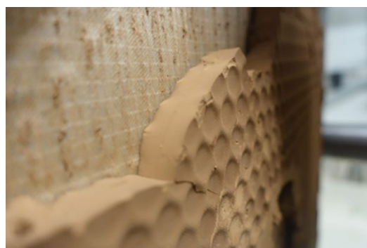
Figure 14 Dried lignin produced from wood chips with the new UNRAVEL fractionation process. ©MVerges UNRAVEL
